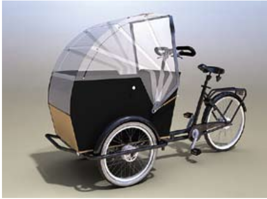
Figure 2: the design of the carrier bike with a hood, which can be used in varying weather conditions to protect children.
